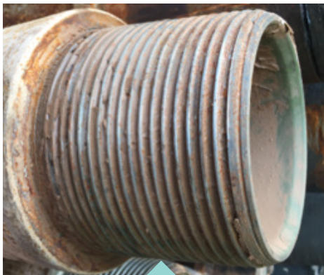
Rag removed from pin connection shows excessive corrosion on 'dry' seal face
