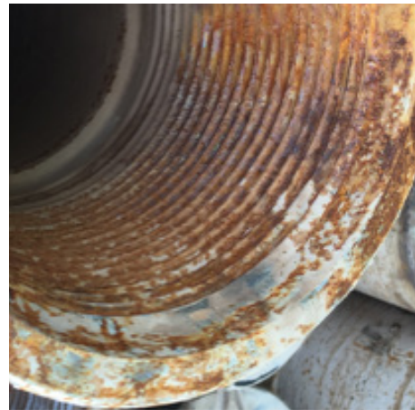
Pipe 'as returned'. Missing protectors and still partially coated with water based mud.
