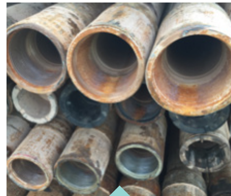
Pipe 'as returned'. Missing protectors and still partially coated with water based mud.
