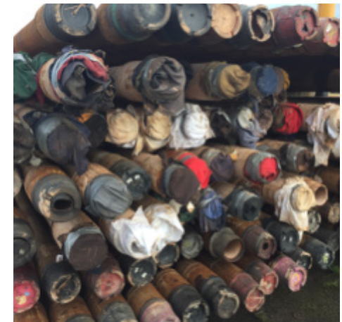
Pipe 'as returned'. Missing protectors and still partially coated with water based mud.
